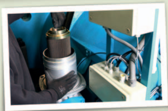
Kidney loop filtration makes frequent oil changes a thing of the past
